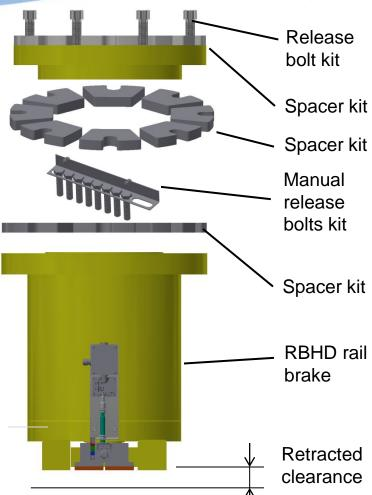
The rail brake spacer kit is provided to ensure that:
